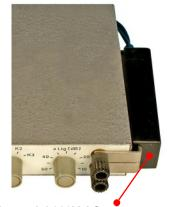
A special 220V AC adapter (German = Lichtnetz Vorschaltgerät), covert number 33604-4/5, was used for a direct connection to AC mains when used with 1st subsystem.
