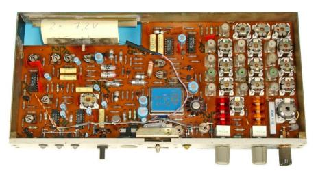
LWE 6-1 with top cover removed showing internal components. Note rows of filters for each of the three channels. A compartment at the top left carried 2 x 7.2V rechargeable batteries.
